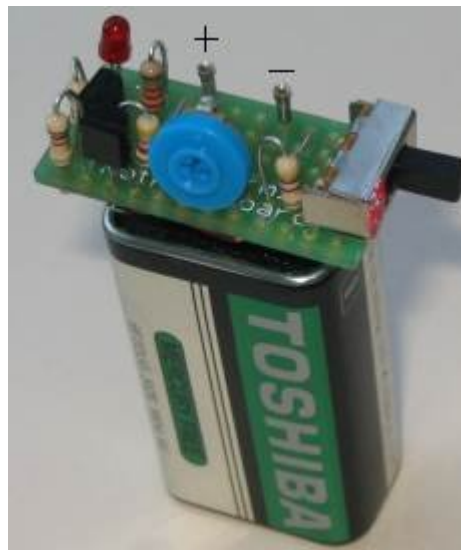
The regulator connected to a 12v battery pack
